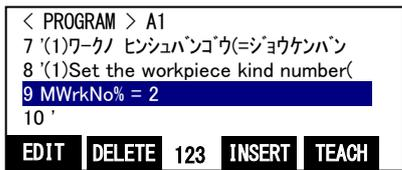
(8) Press the [F1] (FWD) key and execute step feed. "(2)Confirm that Tool is set" is displayed.
