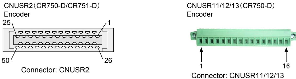
**Figure 12-1 Connector Arrangement**
