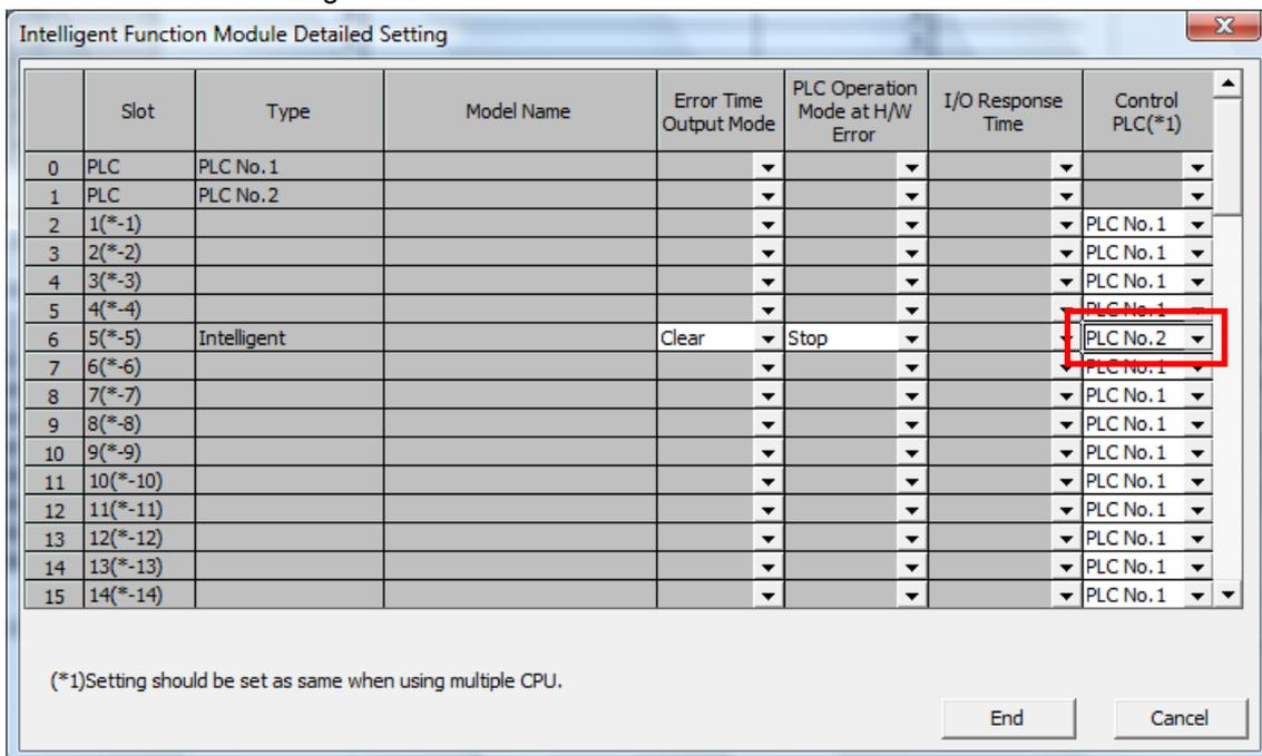
Because the robot CPU manages the Q173DPX unit, change the Control PLC of slot 5 to the “PLC No.2” (Robot CPU).
