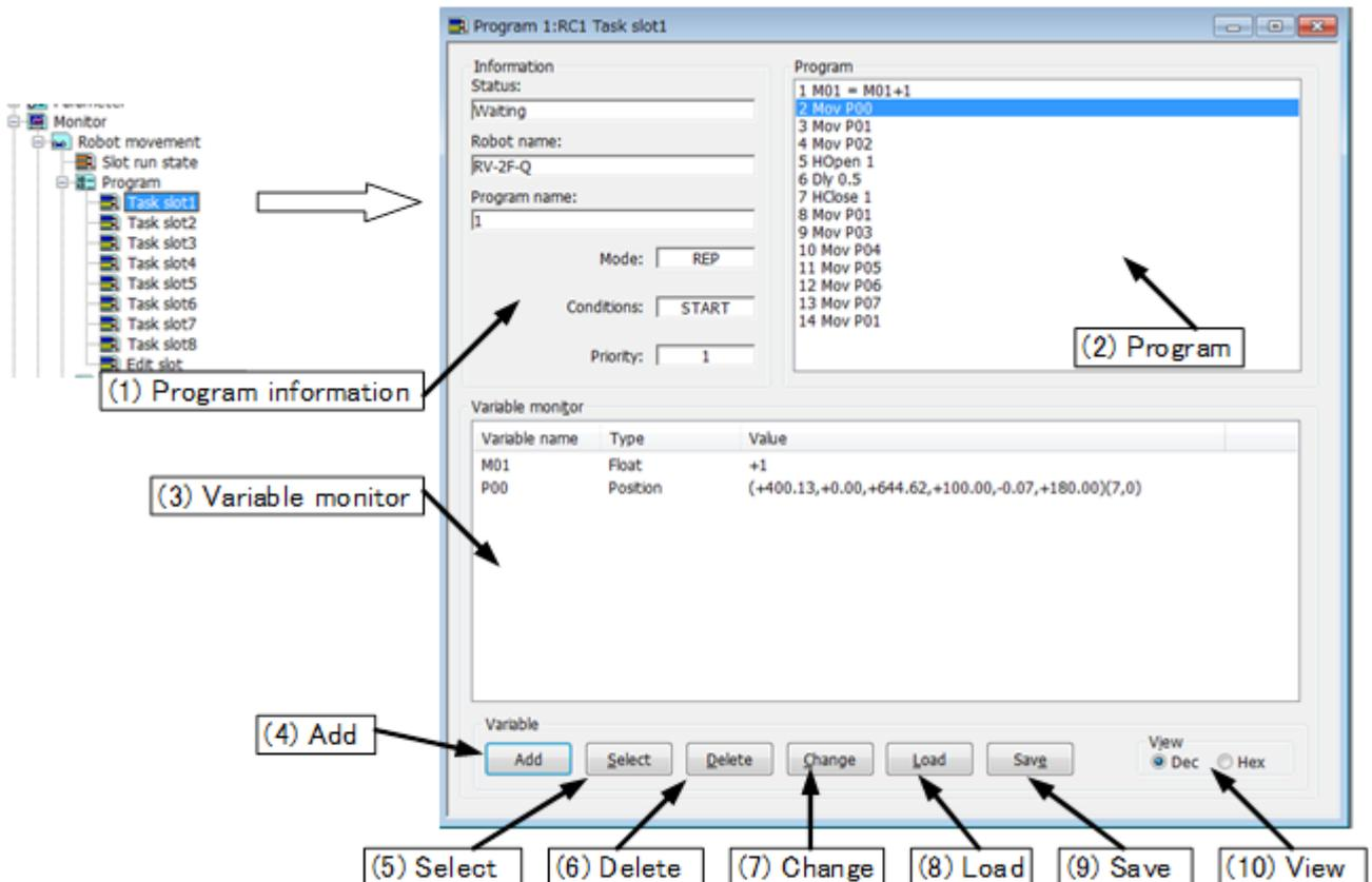
Click a [Add] button and open a "Add display variables" screen. Input "M\_Enc (1)" to a space "variable name", and click a [OK] button. also input "M\_Enc (2)"-"M\_Enc (8)" equally, and click a [OK] button.
