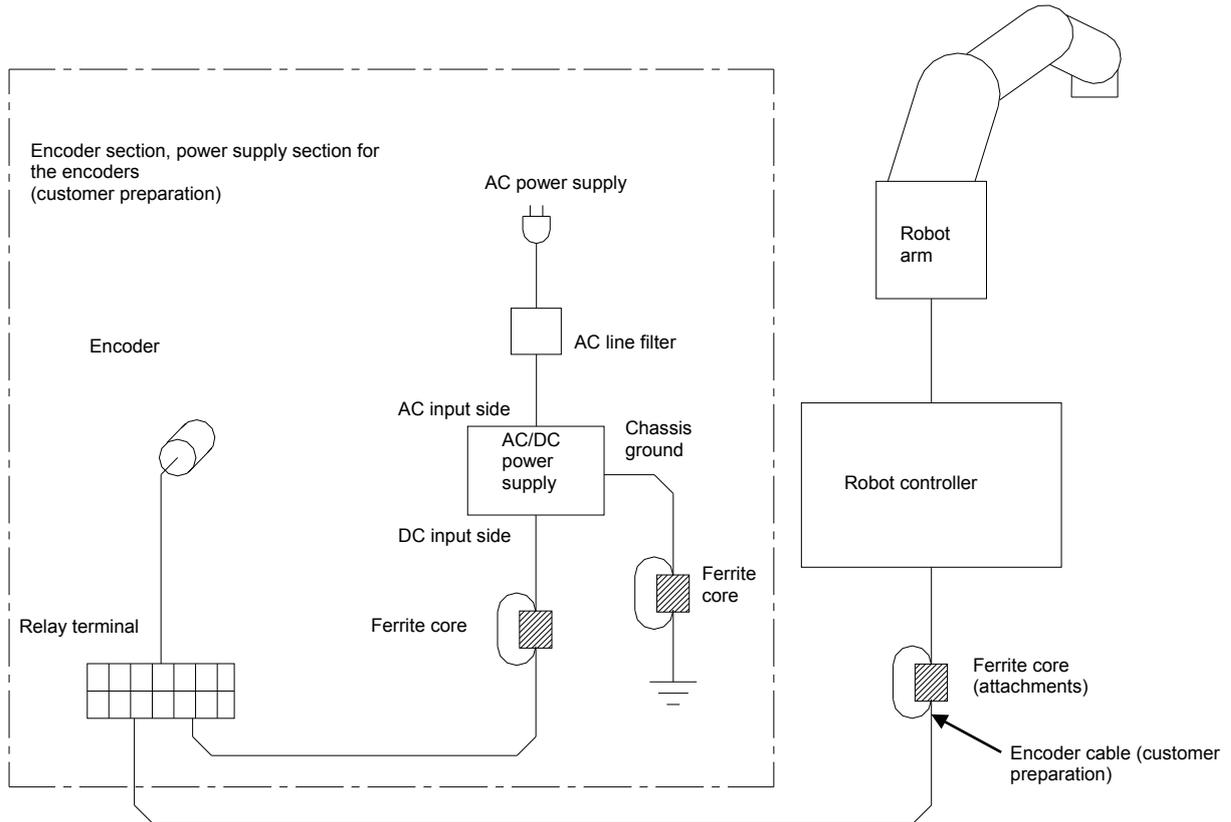
Figure 5-13 Example of noise measures of tracking system
