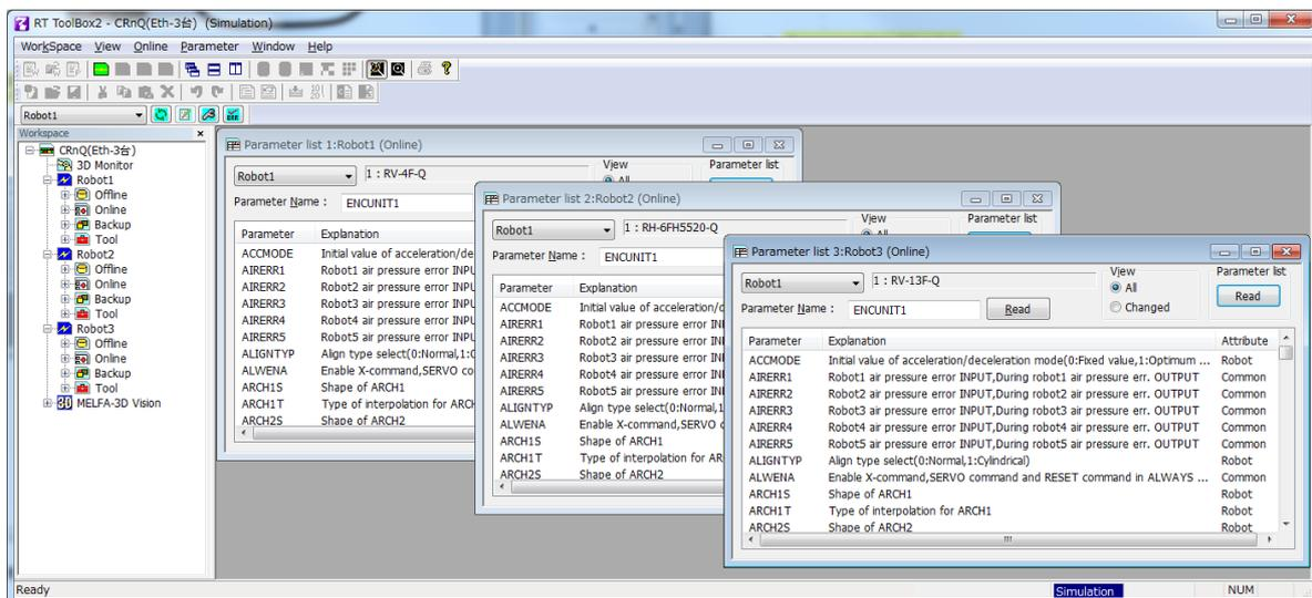
(2) In the setting of robot CPU1 and robot CPU2, specify the value of the parameter ENCUNIT1 to "0,4".
