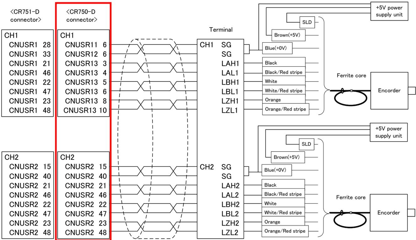
Figure 5-5 The encoder and the wiring diagram of the encoder cable (CR750-D series controller)
