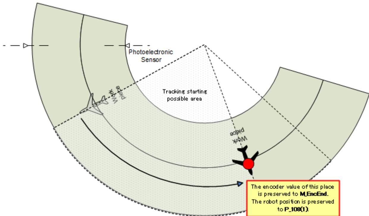
(16) Press the [F1] (FWD) key and execute step feed. "(10)Move the robot to the adsorption point of workpiece" is displayed.
