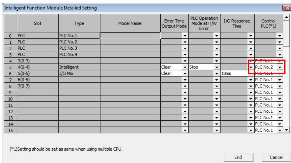
Change “Control PLC” columns to “PLC No.2” in slot 4(0-4) rows of No.5.
