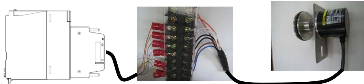
Figure 5-1 Wiring example from an encoder to a unit [Q type]
