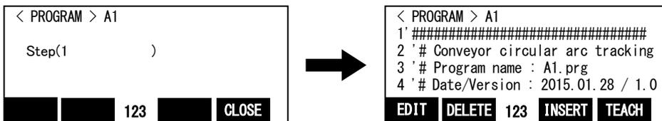
(c) Press the [FUNCTION] key, and change the function display. Press the [F4] (close) key and close the program.
