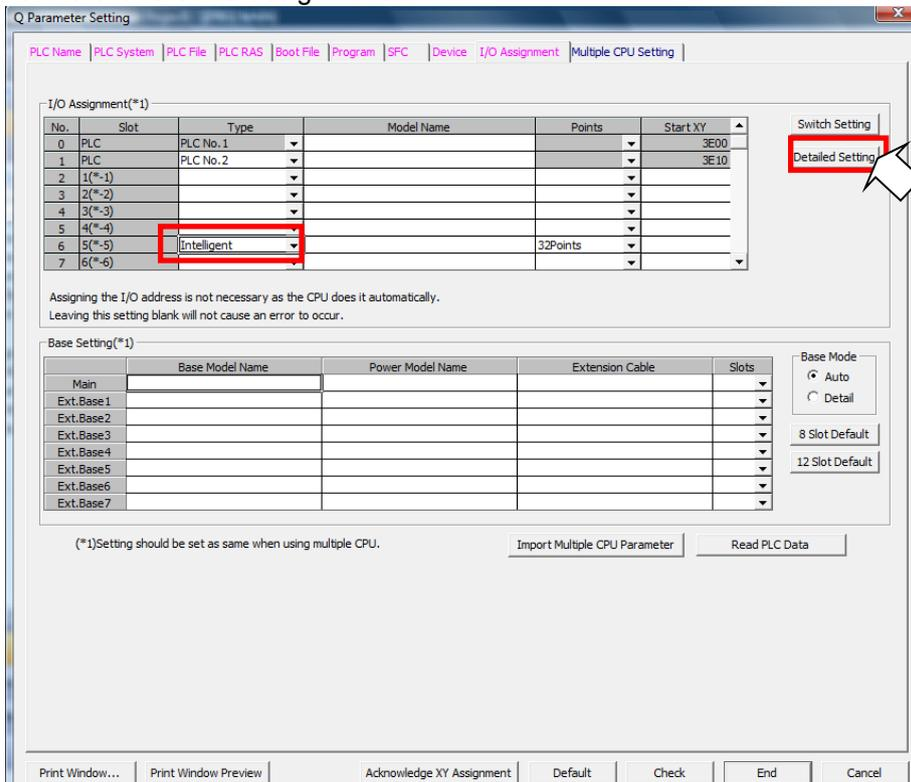
When Q173DPX unit is attached to fifth slot, change the type of slot 5 to the “Intelligent”.
