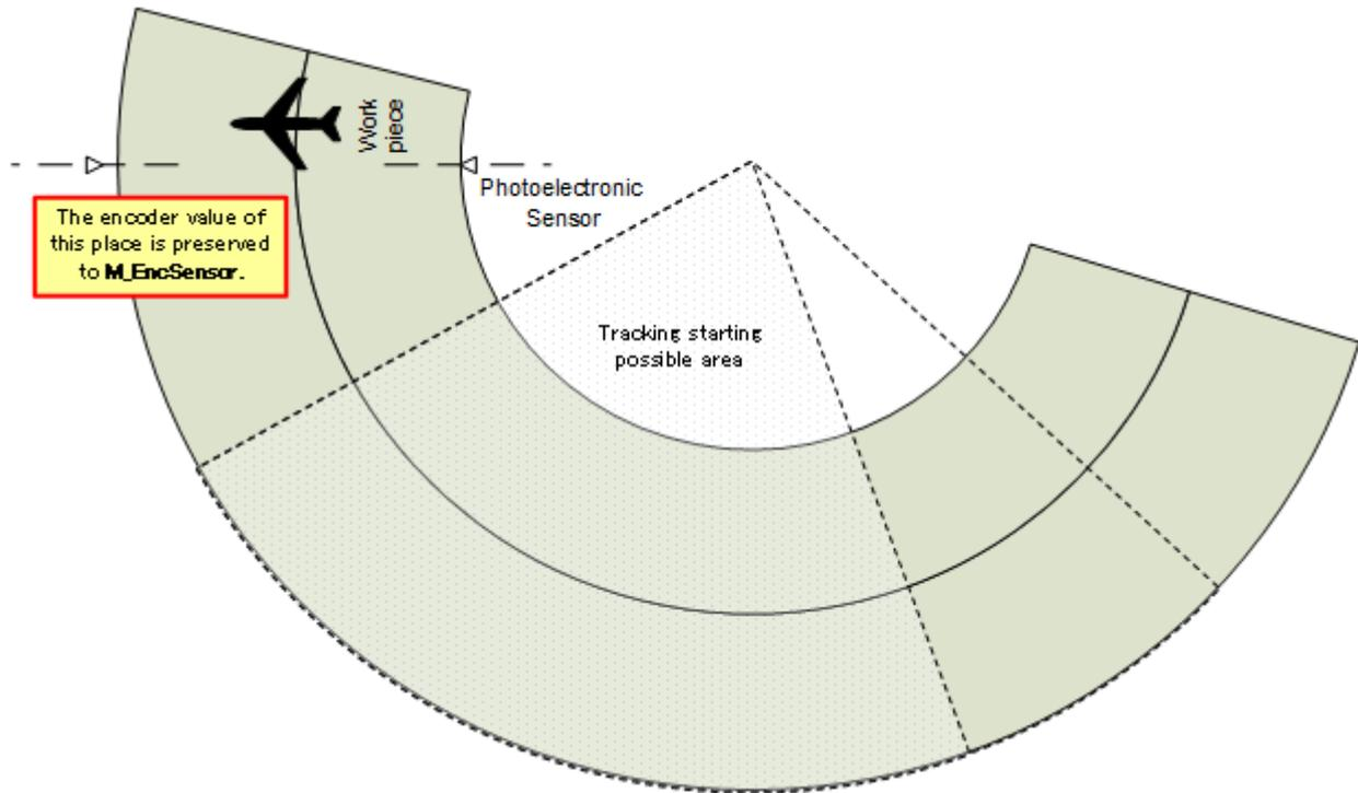
(12) Press the [F1] (FWD) key and execute step feed. "(6)Move workpiece to the tracking area start position by conveyor" is displayed.
