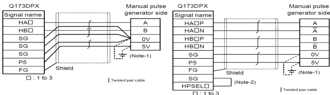
(Note-1) : The 5V(P5)DC power supply from the Q173DPX must not be connected if a separated power supply is used as the Manual pulse generator/Incremental synchronous encoder power supply. Use a 5V stabilized power supply as a separated power supply. Any other power supply may cause a failure.
