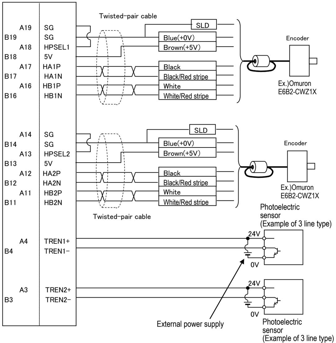
Figure 5-2 The encoder for the conveyor and the wiring diagram of the encoder cable [Q type]
