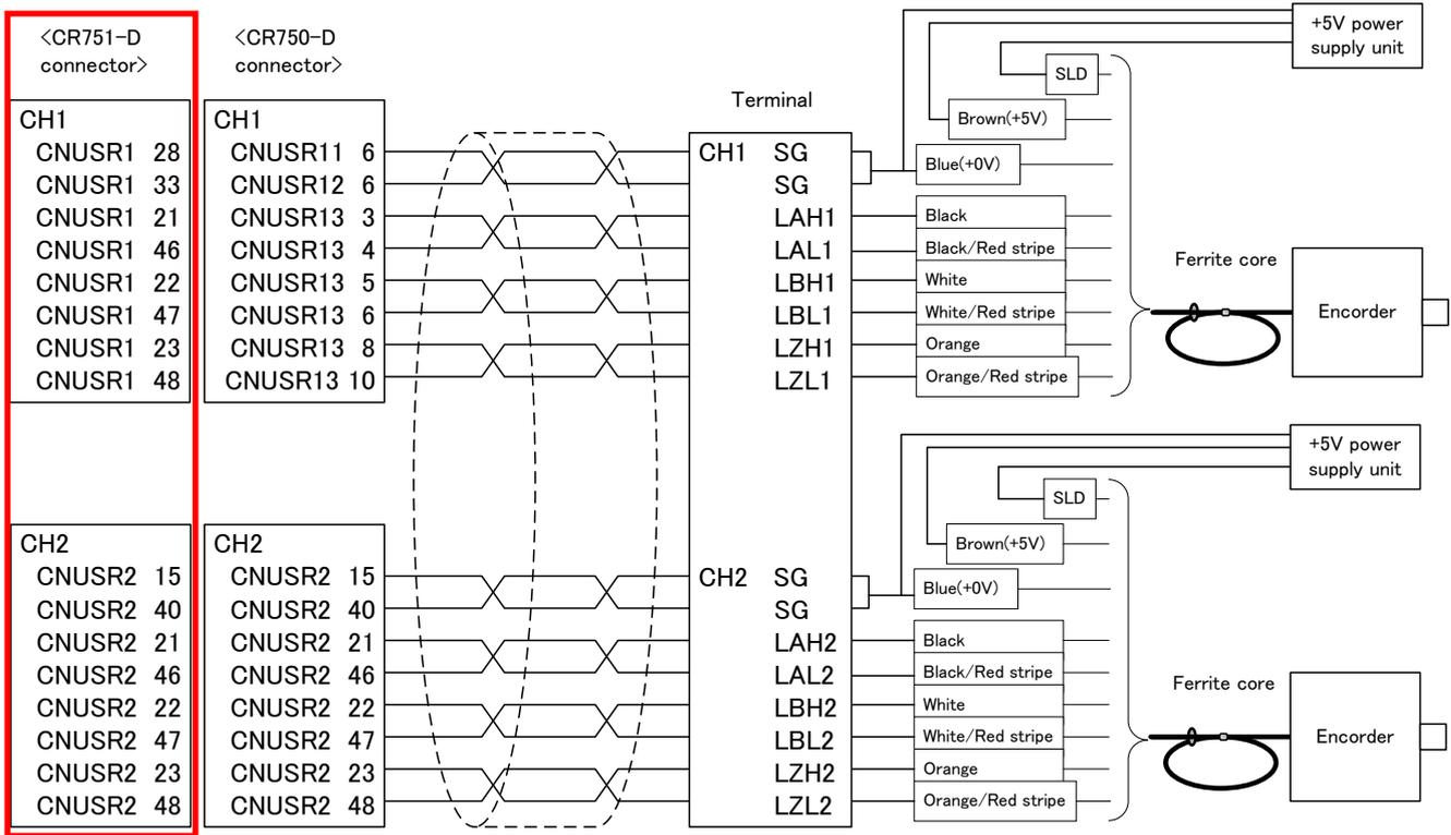
Figure 5-7 The encoder and the wiring diagram of the encoder cable (CR751-D series controller)
