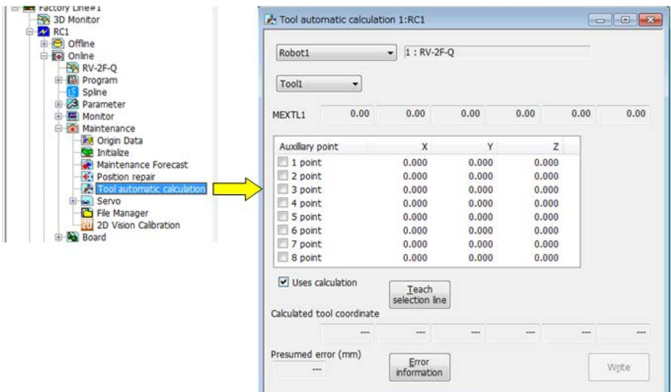
Tool length is calculated automatically by instructing in the location of 3-8 points as follows in the screen mentioned above.
