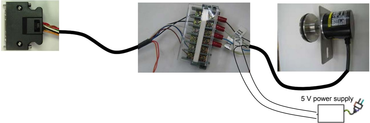
Figure 5-6 Wiring example (CR751-D series controller)
