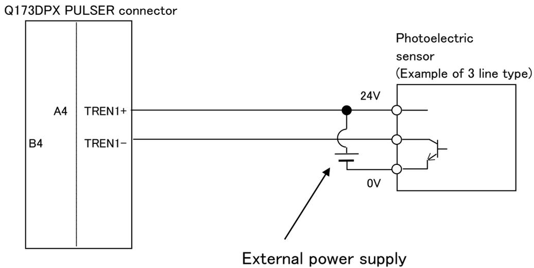
Figure 5-3 Photoelectric Sensor Connection Example (6th General Input Signal is Used) [Q type]
