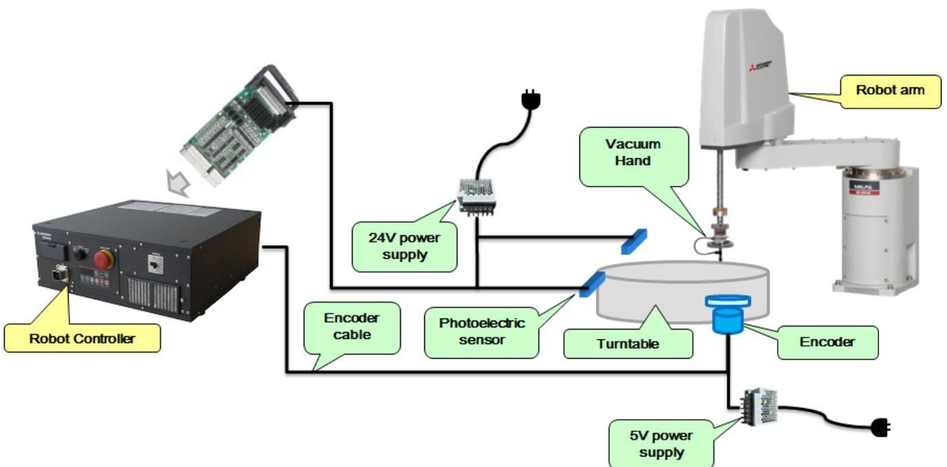
Figure 2-2 Configuration Example of D type
