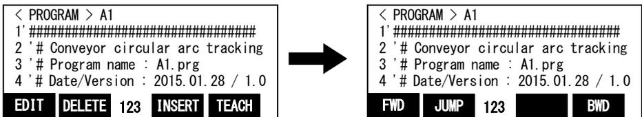
(7) Press the [F1] (FWD) key and execute step feed. "(1)Set the workpiece kind number( = condition number) to the variable "MWrkNo""is displayed. Execute work according to the comment in the robot program.
