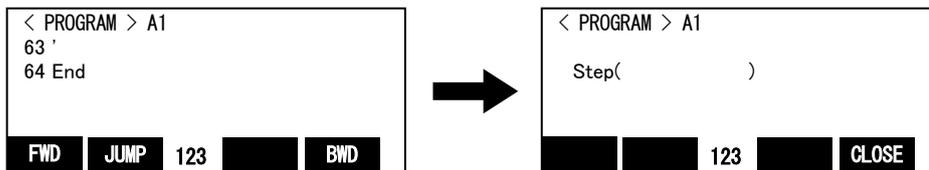
(b) input the step number. Press the [EXE] key. Then returns to first step
